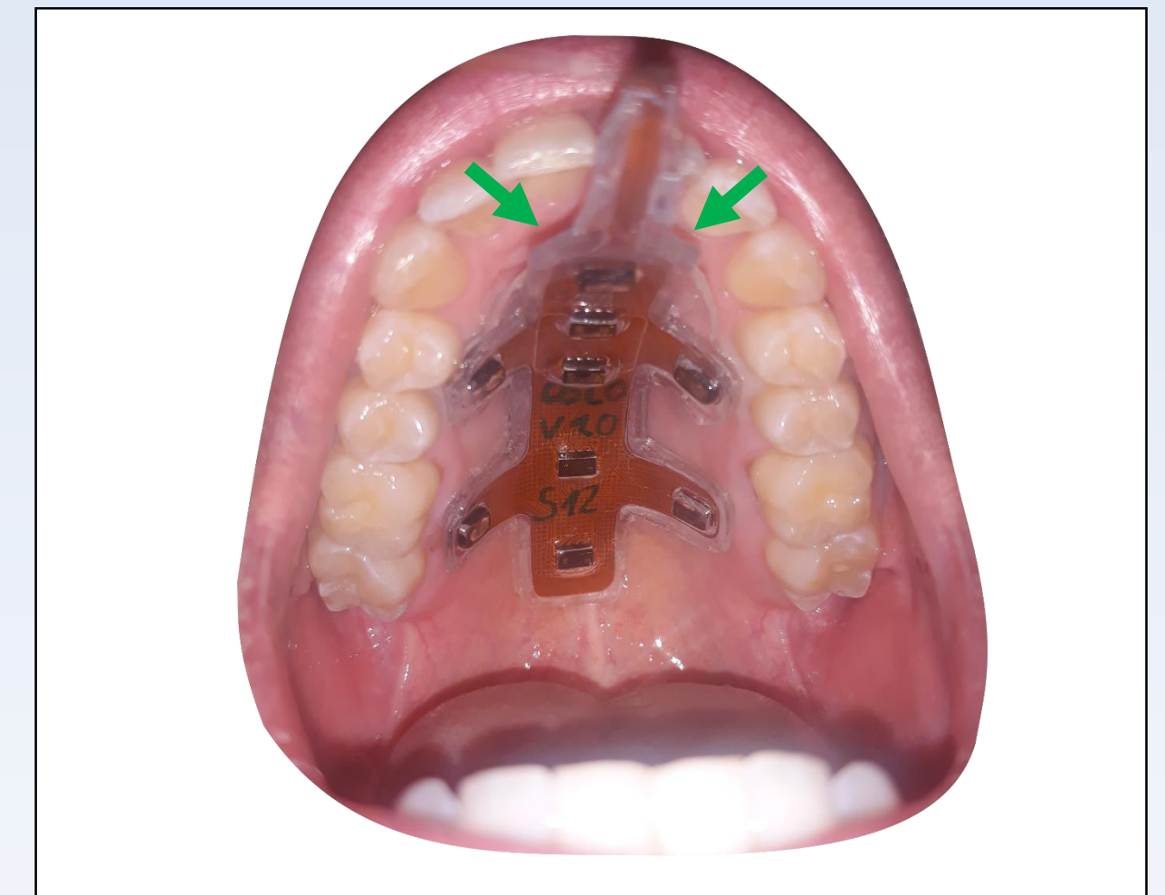
Figure 3: Sensor placement against the hard palate. Green arrows indicate regions of frequent detachment.
